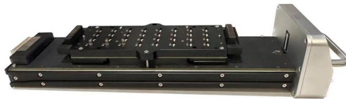
To can fixture and drawer with in-situ front optical power monitor and LIV scan function
